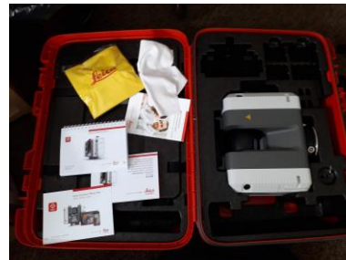
Figure 25: Leica RTC 360 Professional Laser Scanner
