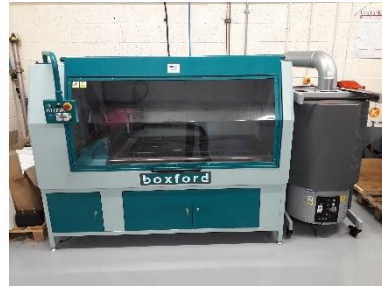
Figure 8: Plasma Cutter - Boxford A1HSPi – 80 Amp
