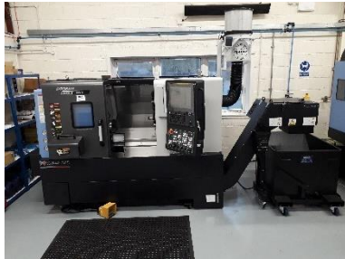
Figure 7: Lathe - Doosan Lynx 2100LMB with Fanuc OiTF Plus control
