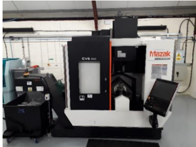
Figure 5: 5-Axis Mill - Mazak CV5-500
