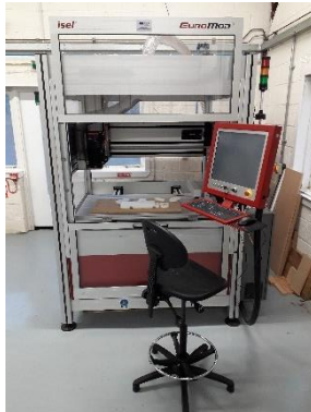
Figure 9: Router - Isel EuroMod MP65
