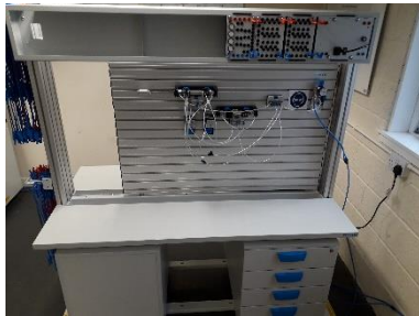
Figure 13: FESTO Double Sided Mobile Pneumatic Workstation
