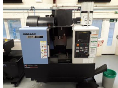
Figure 6: 3-Axis Mill - Doosan DEM 4000 with Fanuc OiMF control
