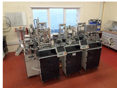
Figure 16: FESTO 8 Station Industry 4.0 Modular Learning System + AGV
